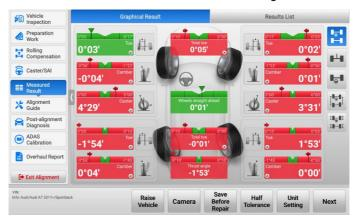
Figure 5-66 Measured Result (Full Tolerance) Screen
