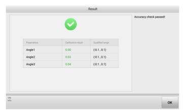
Figure 5-56 Quick Accuracy Check Result
