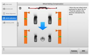
Figure 6-40 Wheel Rolling Compensation 1
