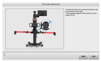
Figure 5-10 Roll Angle Adjustment 2
