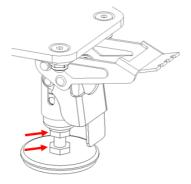
Adjustment method: use 2 monkey wrenches to snap into the two nuts on the bottom of the footbrake and loosen the upper nut in a clockwise direction, then rotate the foot cup to adjust to a suitable height. After that, rotate the upper nut in an anticlockwise direction to tighten the footbrake.
