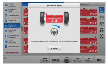
Figure 5-63 Save Before Repair Screen 1
