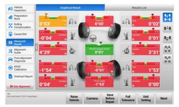
Figure 5-65 Measured Result (Half Tolerance) Screen
