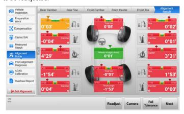
Figure 4-57 Alignment Result Screen
