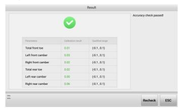
Figure 5-40 Accuracy Check Result Screen
