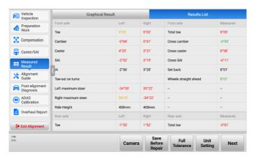
Figure 4-54 Measured Result Screen (Results List)
