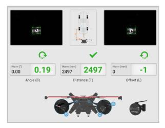
Figure 6-44 Position the Calibration Frame
