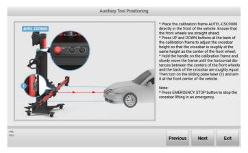
Figure 5-53 Auxiliary Tool Positioning 3
