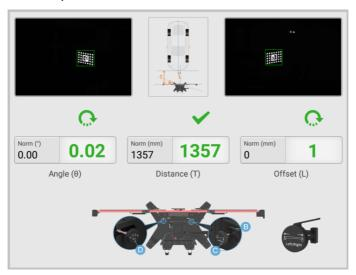
Figure 6-7 Adjust the Calibration Frame
