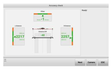
Figure 5-37 Accuracy Check Screen (Use Calibration Bar) 3
